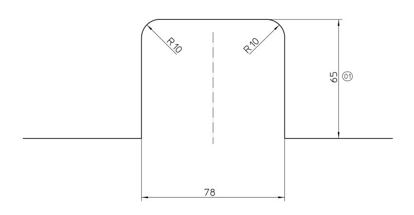
fuer 10 mm und 12 mm ESG for 10 mm and 12 mm toughened safety glass
