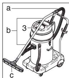
☞ Wrap the power cord (9) completely. Install the required accessories (eg water suction (c)).
