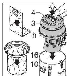
☞ Switch off vacuuming (3). Open the tank clips (10) and take out the motor bonnet (4).
