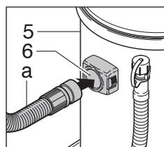
☞ Suction hose (a) in the hose connection (6) to the boiler (5) connect.
