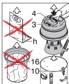
☞ Switch off vacuuming (3). Open the tank clips (10) and take out the motor bonnet (4).
